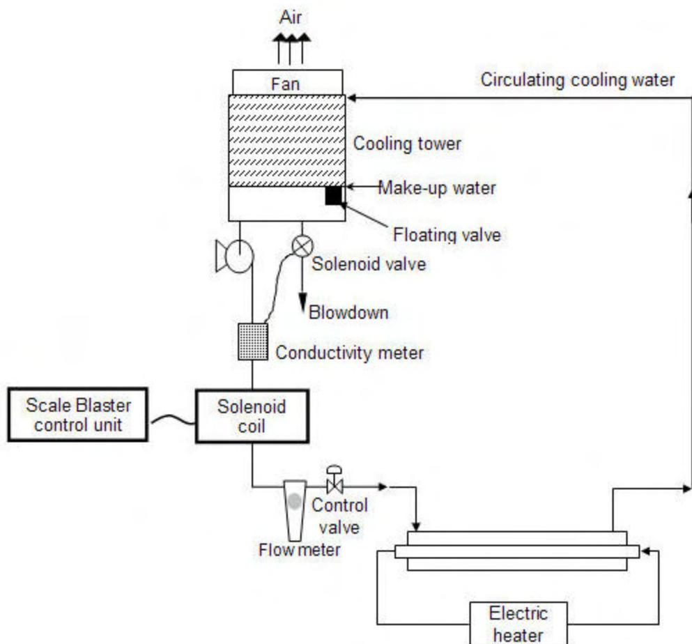
This system deviated from the ASHRAE protocol in that a tube-in-tube heat exchanger was used instead of a flat plate heat exchanger as in the case of the ASHRAE protocol.
