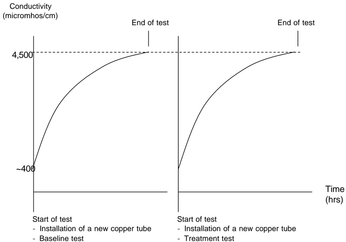
The above figure represents the electric conductivity regime utilized for this test. This study was a “no-blowdown” test, which provided a more aggressive water chemistry than using conductivity setpoints. Well-water in Phoenixville, Pennsylvania had a conductivity of between 400-450 micromhos/cm, and through evaporation, was cycled up to 10. Bio-control was conducted by adding 0.5 ounces of 15% glutaraldehyde solution into 10 gallons sump water daily.
