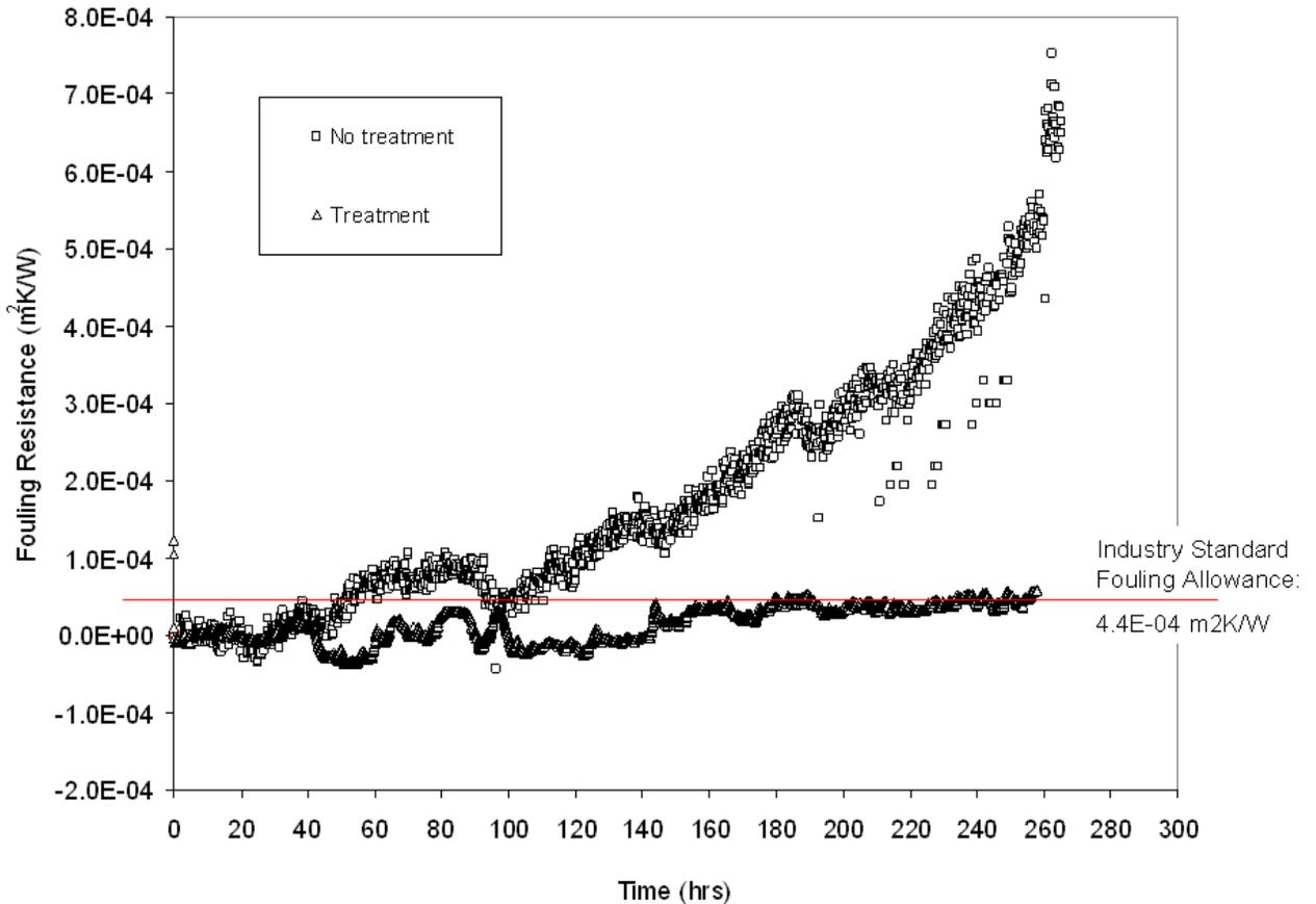
After 11 days, the Baseline test achieved asymptotic values of fouling resistance, whereas the Scale Blaster was able to keep the fouling resistance at below the industry-standard clean values, approximately zero or negligible fouling after the same amount of time as the Baseline and all other conditions held equal.
