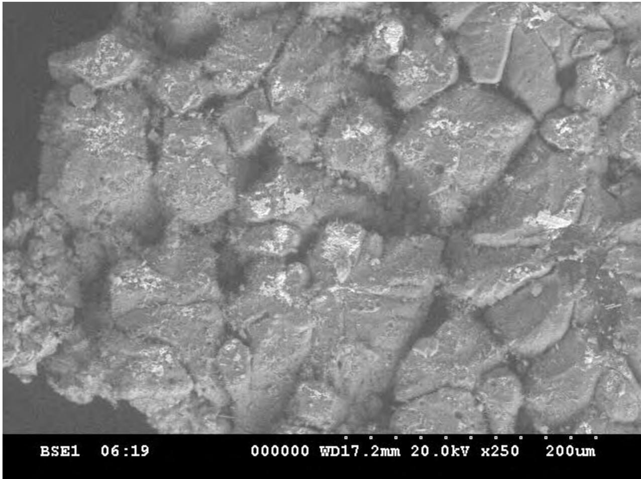
The above image was taken of dried deposits of Baseline test deposition using an SEM camera at 250x magnification. The image of scale seen is typical calcite formation having the granular composition of crystallization fouling.
